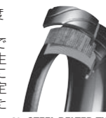
0°- STEEL BELTED TYRE WITH RADIAL CARCASS (90 DEGREES)
