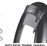
BELTED TYRE WITH RADIAL CARCASS (90 DEGREES)
